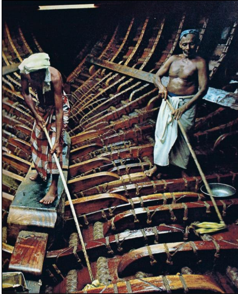
Oiling down the inside ribs of the hull
